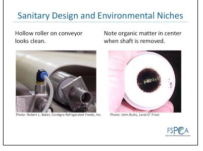
Sanitary design is an important consideration to prevent product contamination. An example of a potential source of environmental contamination is the hollow roller on a conveyor illustrated above. The equipment looks clean but when the shaft is removed, organic matter that can support microbial growth is evident in the center of the roller. This type of site may be impossible to clean and sanitize with a normal cleaning procedure.
