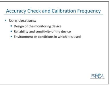
It is important to realize that the accuracy of monitoring devices can change, therefore it is important to conduct routine accuracy and periodic calibration checks to assure safety and to minimize the need to detain and evaluate product. A number of factors should be considered when determining the frequency of these activities for monitoring devices.
